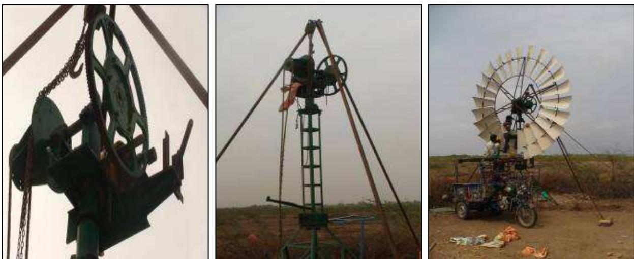
During the dry span of the rainy season, we did the trials to measure the performance of the power generating windmill. Ammeter, voltmeter, 24 volt battery and anemometer are the instrument used to collect readings.
