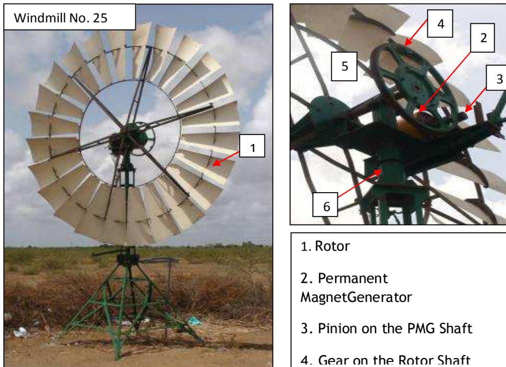
The power generating windmill has been installed using the three poles and chain pulley system. The following pictures shows the installation process,
